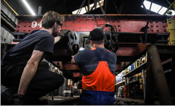
Left: Hamish and Dave removing 945's tender drawgear for inspection and non destructive testing. Right: ORB #2 pulls 398 out of the shed during a re-shuffle, this is the first time since November 2011 that the locomotive has seen the outside.
