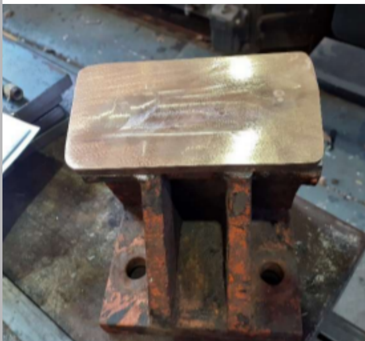
Left: Chafing block with bronze packer. Right: The chafing blocks fitted to the trucks
