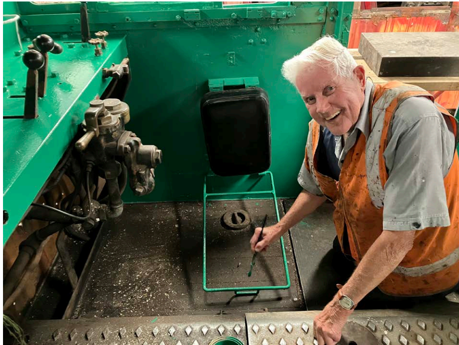
Ron Jones applies a finishing green enamel to the cab interior and fittings of ex-Ohai Railway Board diesel loco #1, a precursor to the Ds class. Photos: RIR
