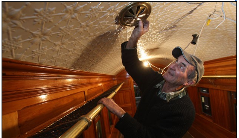
FINISHING TOUCHES: Pleasant Point Museum and Railway volunteer Bill Noble at work on the new aluminium panel ceiling inside the 1912 carriage.
