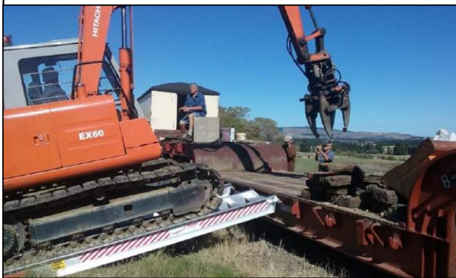
Left. Nice Engineering Solution. Gary Kelly tries out the new digger loading ramps that were funded thanks to a grant from the Mainland Foundation. The new ramps will allow easier and more convenient access for our digger along the line. 24th of February, 2016. Photo: Maurice Fenton.
