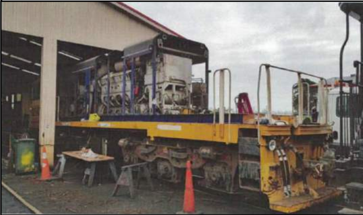
DBR 1254 has had much of its Long Hood and sundry equipment removed to assess condition of the frame. Photo from YARN
