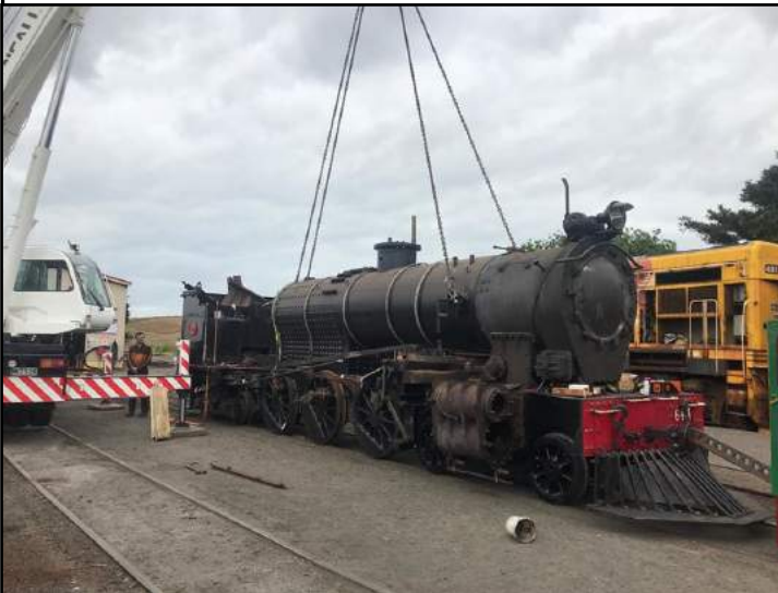
Meanwhile back at the workshops at Pukeowhare much work continues. Lifting the new boiler onto Ww 644. DC 4818 in the process of disassembly sits in the sun.
