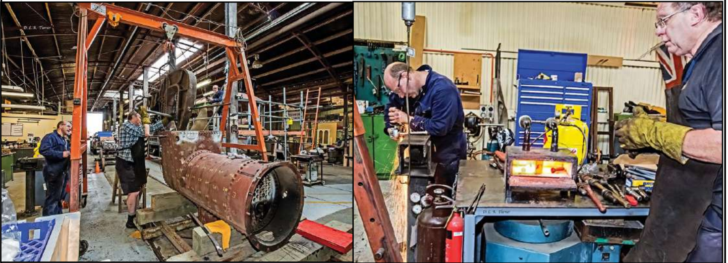
Above left: Gap Riveting Kitty's Replacement Boiler. Removing a temporary fastening bolt, a length of pipe providing the necessary extra leverage.
