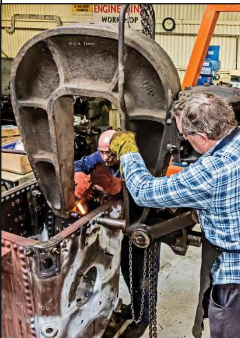
Above: Alex Hunter delivers a molten rivet to Allan Famliton operating a Gap Riveter.
