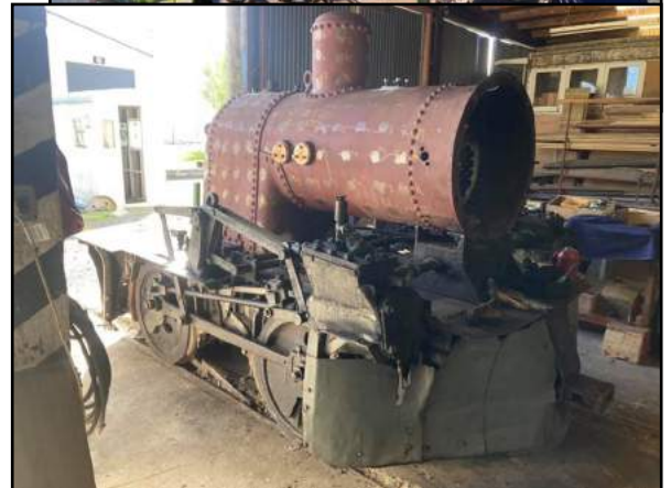
Above Left: September 19. The body has been removed to enable the old boiler to be lifted out. Photo: Stephen Taylor.
