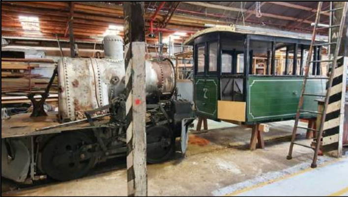
Above Left: September 19. The body has been removed to enable the old boiler to be lifted out. Photo: Stephen Taylor.
