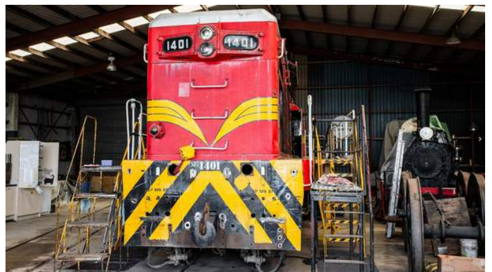
DA1401's headstock following removal of the cowcatcher
