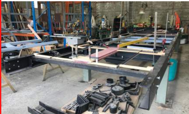
Left: Reassembly of tram 207's renovated and repainted chassis is underway at Tram Works Ltd's workshop in Otahuhu.
