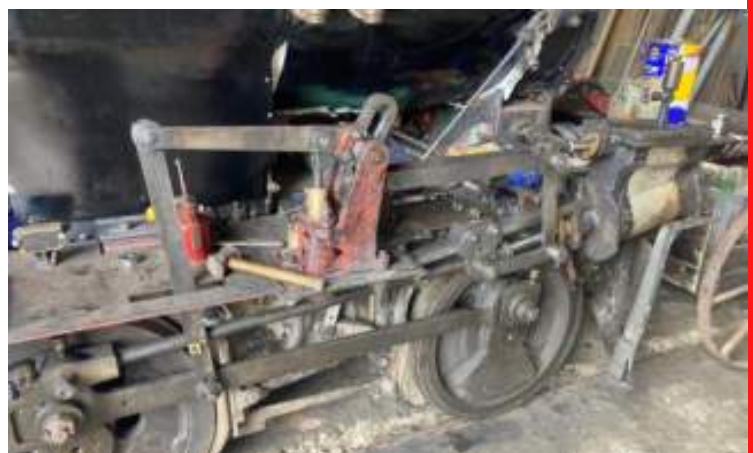
Left: Body work with the side off ready for paint preparation. Right: The RH Valve gear all assembled and ready for setting up. Photos: Ferrymead Tram Facts
