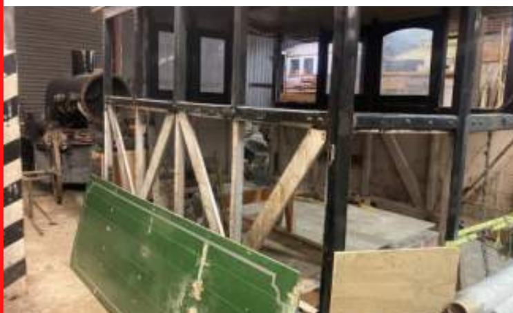
Left: Body work with the side off ready for paint preparation. Right: The RH Valve gear all assembled and ready for setting up. Photos: Ferrymead Tram Facts
