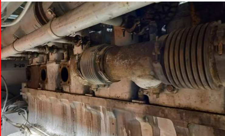
Left: Short branch exhaust and water outlet rail assembled. Right: Final assembly completed. Photos: DTG Facebook
