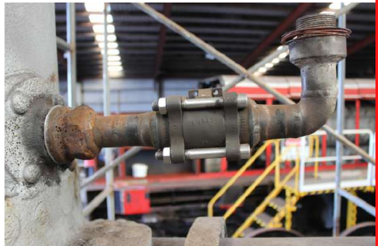
Left: DA1401 sits inside the engine shed. Right: The old pipework was removed from the whistle of WAB794, with new pipework including a shut off valve being installed (as pictured). Photos: Letting Off Steam
