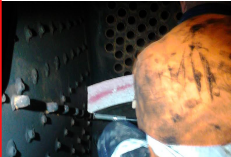
Left: WA165 fitting the fire bricks, right: DSC2759 Brake Caliper Servicing. Photos: Graeme Scott
