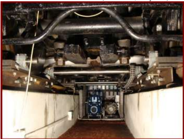
Underside of H199 showing centre rail brakes and drive wheels. Featherston, (Nigel Hogg, 7 June 2010)
