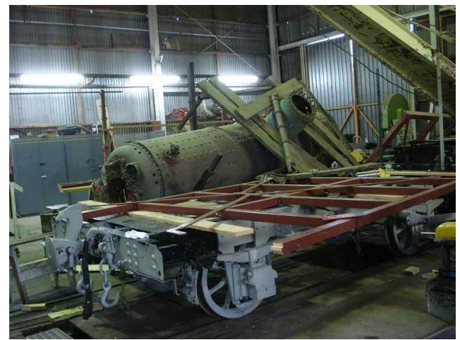
Pictured is F13's boiler which survived a fall off its stands. Photo : Flugel.
