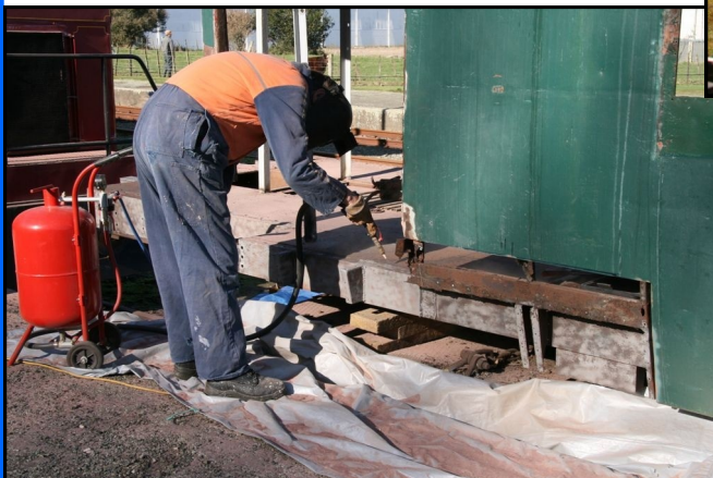
Lee Hall sandblasting the cab floor structure. Photo: Doug Johnston
