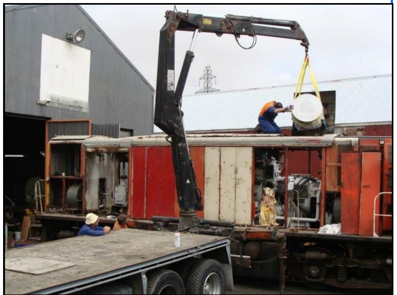
The work continues. Refitting the turbo-charger to DI 1102, Feb 2012
