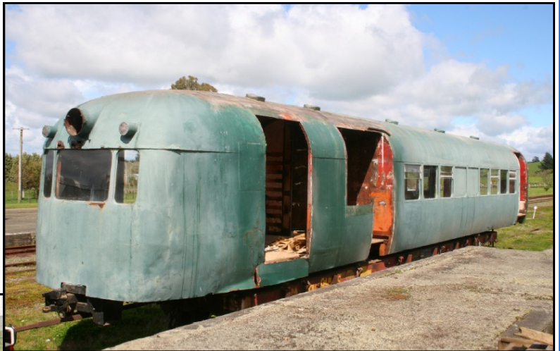
RM 121 No 1 end car during the strip out and removal of modifications, October 2011; Photo: Doug Johnston
