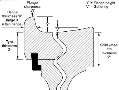
(a) When wheels are turned profiles must conform to NRSS 6; Clause 8.2 and Appendix A.  $^{6}$
