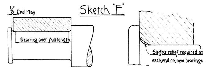
When fitting bearings to the axle journal it is desirable to have as much bearing area as possible so that the pressure per square inch of the area in contact, due to the load, may be
