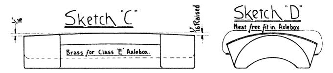
This type of brass should not bear against the box over the full length at the back, but it must be a close free fit sideways.
