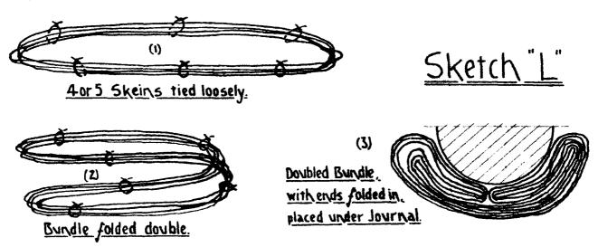
Also, when yarn packing is used it should not come above the centre line of the journal. The yarn packing should be keyed at the front of the box by means of a tightly wound bob.
