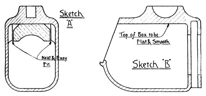
The end play of the bearing in the axlebox should be from 1/16" to 1/8".
