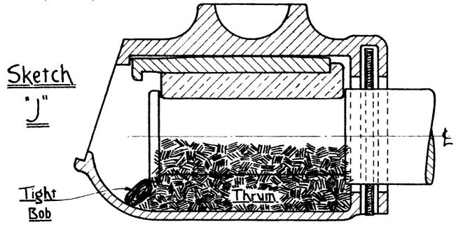
Wool packing as used in axleboxes must be carefully prepared before it is put into use.
