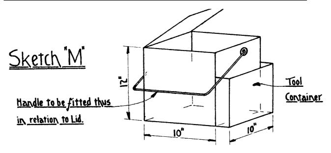
The bucket provided for carrying packing should be used solely for that purpose; tools such as hammers, chisels, scrapers, small bottle jacks, etc., should not be carried in with packing, but in the compartment provided, or in some separate small bag or container.
