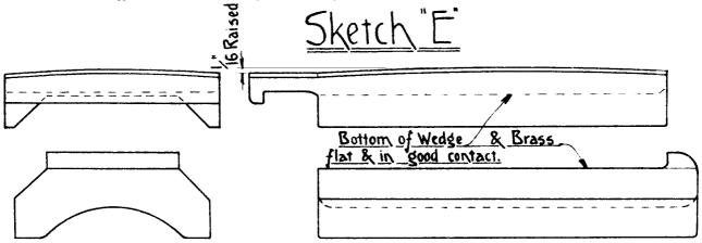
This roll allowed between axlebox and bearing (or wedge) is essential so that when any jar or rough riding tends to cause the axlebox to cant endways, the bearing will maintain full and even contact over the whole length of the journal, while the axlebox can roll on the back of the bearing (or wedge). This is most important when axleboxes fit neat in the horns.
